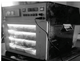
Fig. 7. 50 embryo capacity computer controlled incubator with a visible light ovoscope.
